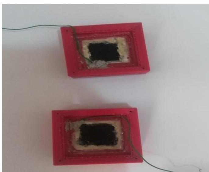
Figure 4: Fabricated Zinc-air mechanically rechargeable batteries
