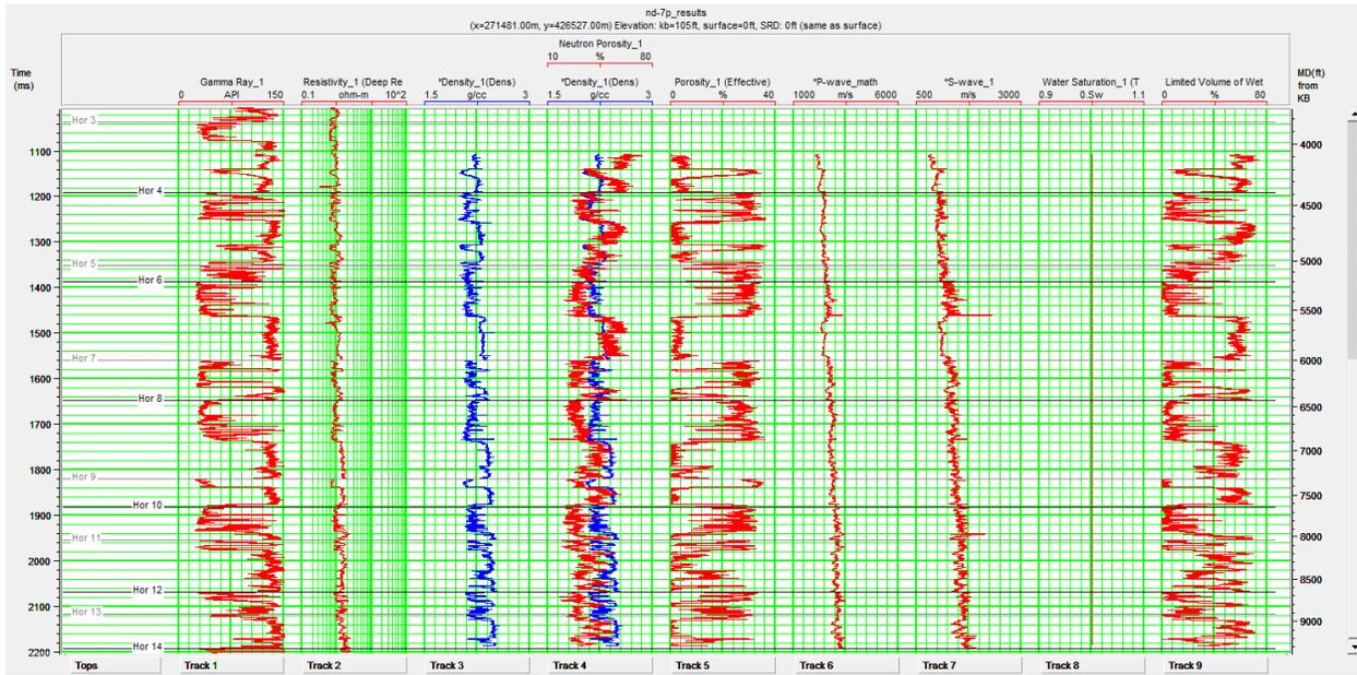
Figure 1: Well Nd-7p showing some selected logs with well tops. Track 1: Gamma log, Track 2: Deep resistivity, Track 3: Density, Track 4: Density (blue) and Neutron log (red), Track 5: Effective porosity, Track 6: P-wave, Track 7: S-wave, Track 8: Water saturation, and Track 9: Volume of shale/clay.
