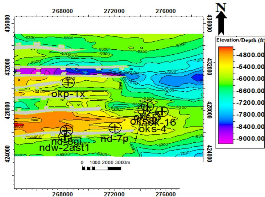
Figure 4: Depth structure map for reservoir Hor 7 showing fault polygons, fault-assisted closure and four-way closure
