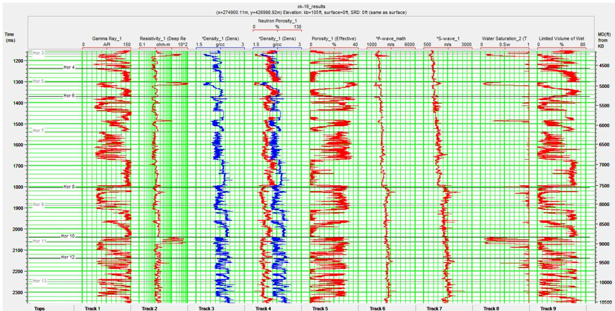
Figure 2: Well Ok-16 showing some selected logs with well tops. Track 1: Gamma log, Track 2: Deep resistivity, Track 3: Density, Track 4: Density (blue) and Neutron log (red), Track 5: Effective porosity, Track 6: P-wave, Track 7: S-wave, Track 8: Water saturation, and Track 9: Volume of shale/clay.
