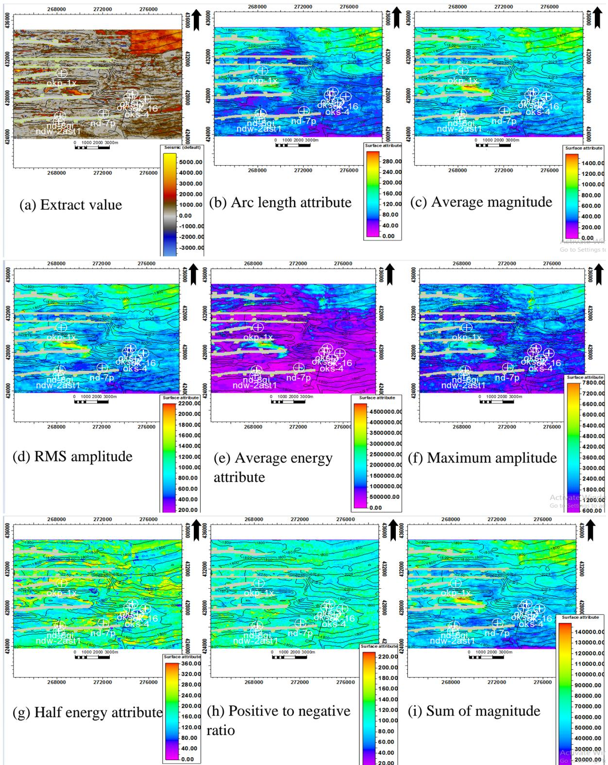
Figure 5: Surface attributes extracted around reservoir Hor 7 within time window 1500 – 1875ms, showing promising regions, red=highest amplitude and purple=lowest amplitude region. The anomaly strength seem to be reduced in both ‘Average energy’ (Figure 5e) and ‘Maximum amplitude’ (Figure 5f) maps around these regions indicating accumulations of hydrocarbon. Those identified regions are porous as
