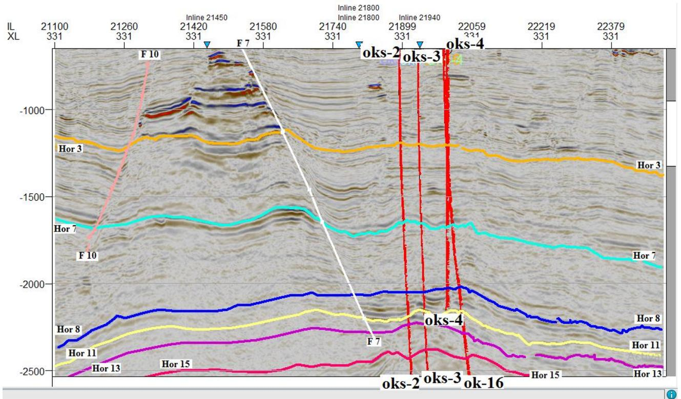
Figure 3: Seismic section showing interpreted reservoirs, well positions and Gamma Ray log (Red) along cross line 331 showing growth fault and collapsed crestal structures.
