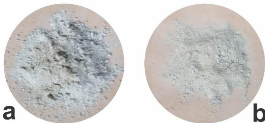
Fig. 5: (a) The milky appearance of Kalambaina Limestone showing microcrystalline calcite with coarse grains. (b) Milky Kalambaina Limestone with microcrystalline calcite, other mineral constituents with fine grains..
