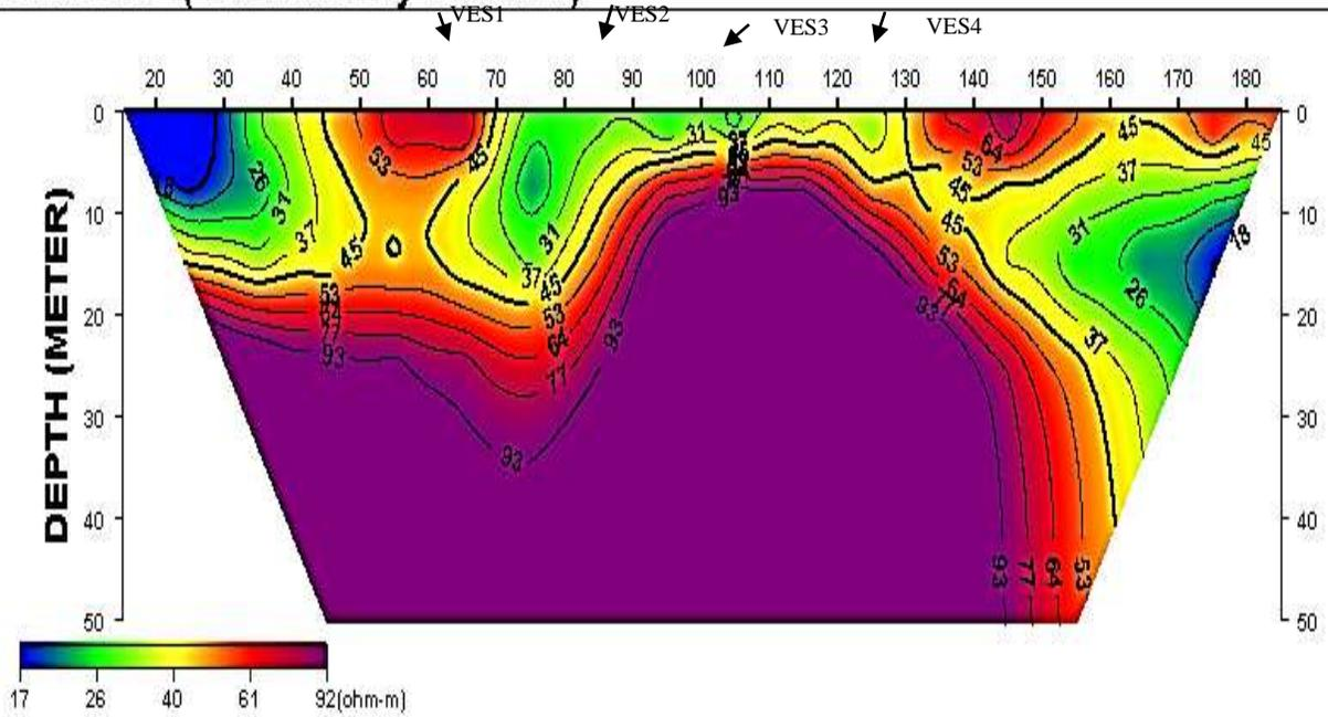
**Figure 5a:** 2D Resistivity Structure (Traverse One)
