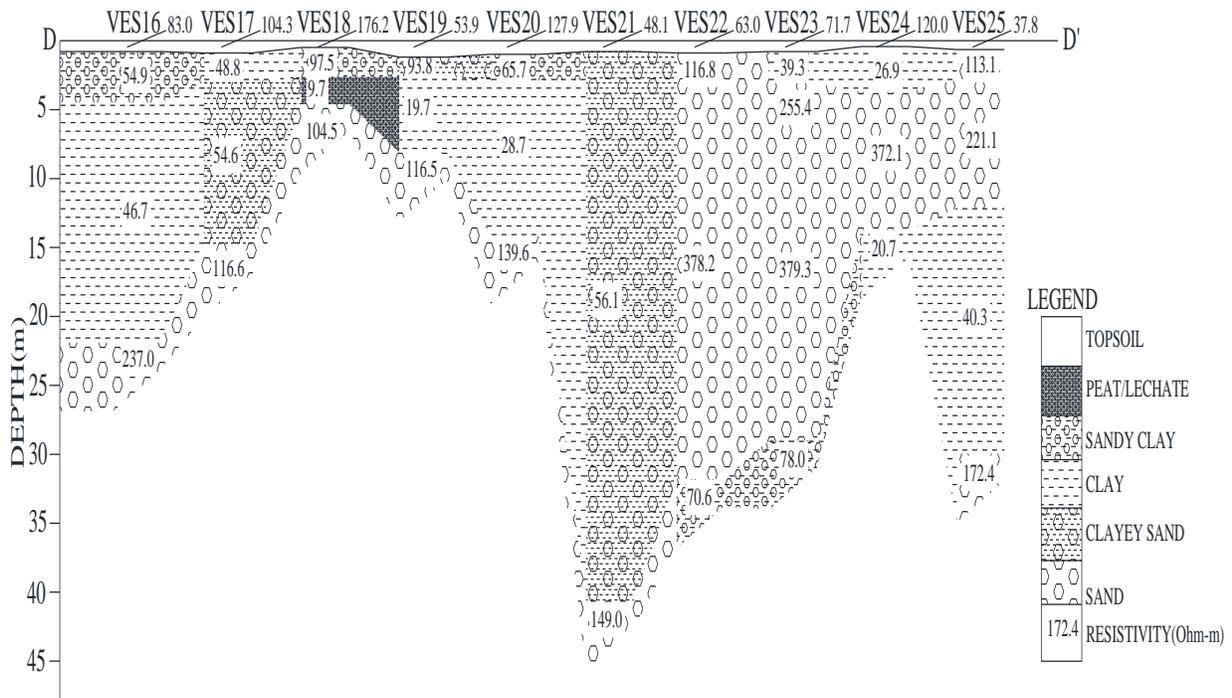
Figure 4d: Geo-electric Section for VES 16, 17, 18, 19, 20, 21, 22, 23, 24 and 25
