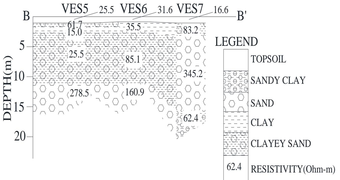
Figure 4b: Geo-electric Section for VES 5, 6 and 7
