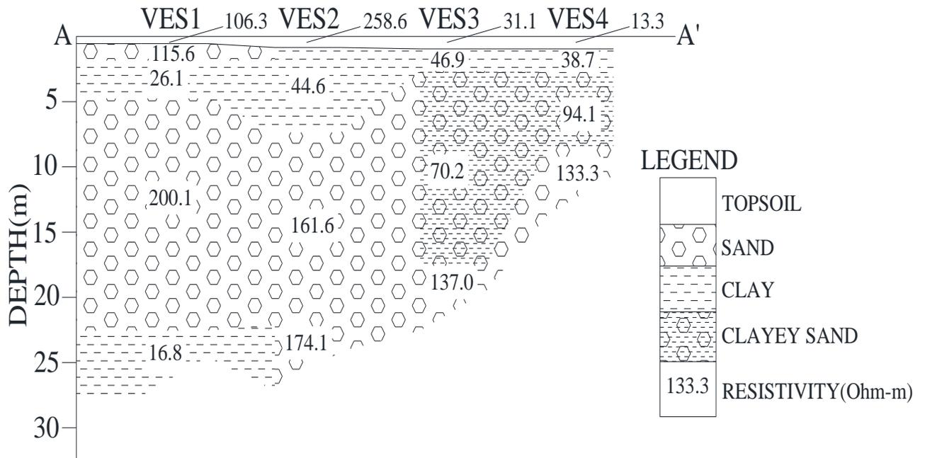
Figure 4a: Geo-electric Section for VES 1, 2, 3 and 4
