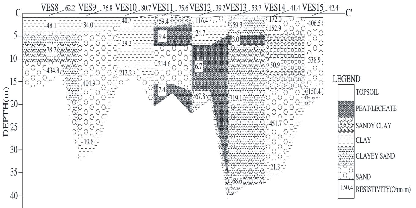
Figure 4c: Geo-electric Section for VES 8, 9, 10 11, 12, 13, 14, and 15
