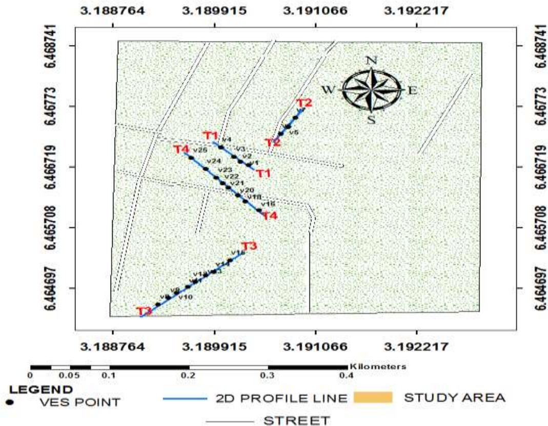
**Figure 3:** Base map survey layout showing the VES stations and lines of transects for the ERT profiles
