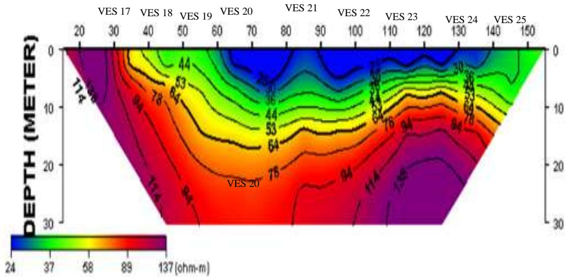
Figure 5d: 2D Resistivity Structure (Traverse four)
